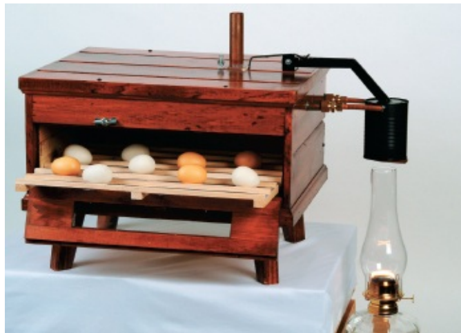
This 50-egg kerosene incubator from Lehman's uses an oil lamp to heat water that circulates in copper tubing to maintain a constant hatching temperature.
